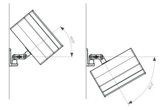
Figure 10. Mounting possibilities in the vertical plane for IC 32 with SMB in the center points.
