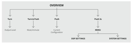
Figure 14. DSP firmware functions and menus.
