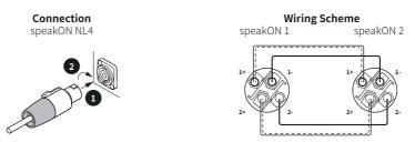
Figure 8. speakON<sup>®</sup> plug-in and link cable connection.
