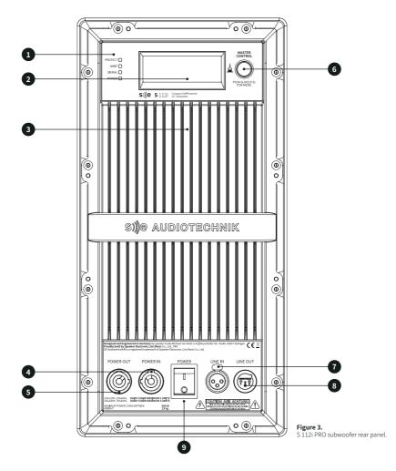
C Line In. Balanced line-level input with female Neutrik® XLR-3 connector to connect input signal. It allows input levels up to +20 dBu.
