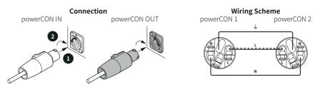
Figure 7. powerCON® plug-in and link cable connection.
