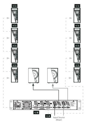
Figure 43. Schematic of Bar or Restaurant Example.
