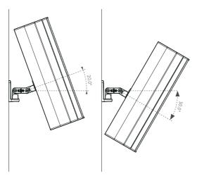
Figure 11. Mounting possibilities in the vertical plane for IC 34 with SMB in the middle mounting position.
