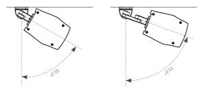
Figure 13. Different aiming angles in the horizontal plane with the SMB bracket.
