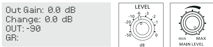
Figure 50. Nominal levels in M-Line subwoofers (left), M-F3A PRO (center) and M-F3A (right).
