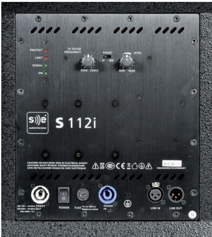
Subwoofer electronics module Level, crossover frequency of the low-pass filter (80-250 Hz) and phase reverse can be set
