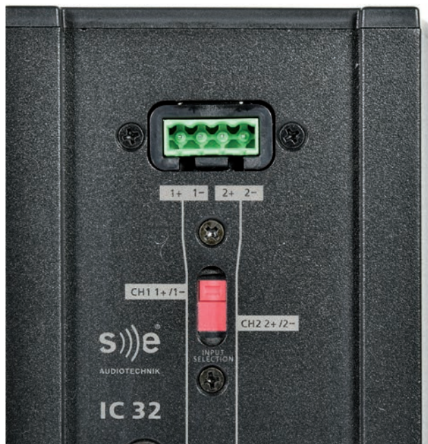
4-pole Phoenix connectors at the top and bottom; users can select via slide switch whether to use signal connections 1± or 2±
